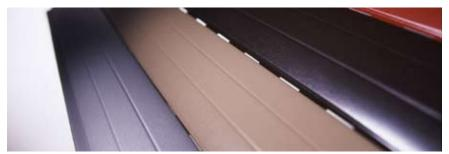
As an alternative to painting finished articles, coil coating provides many benefits because of the efficiency of applying paint by the roller-coating process to flat strip.
